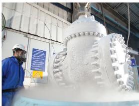
The in-house cryogenic test facility at L&T Valves is one of the largest in the world, built to test valves of sizes up to 60".
