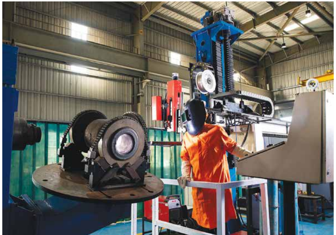
Cladding using Automated Welding Machine
